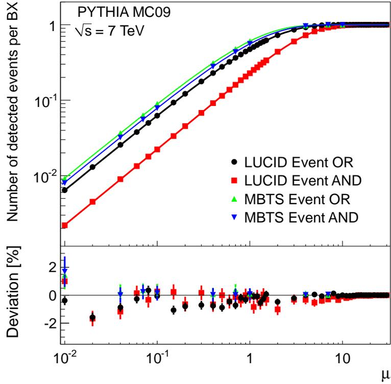
Figure 1: Comparison of probability functions with simulated data. The lines are from the equations and the points from the data. The LUCID OR-counting method is using Equation 8, while for LUCID AND-counting Equation 25 is used.
