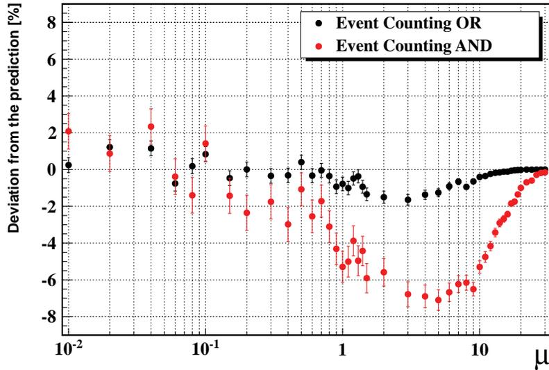
Figure 2: The difference between the simulated data and Equation 8 and 25 when the LUCID threshold is increased to 50 photoelectrons.
